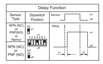
**Note:** It is understood as the sensor activation when the output inverts its state in relation to the rest condition. For instance, PNP (NO) in rest shows the output in "0" and when activated changes for "1".
