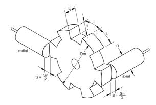
Slotted disc diameter calculation
