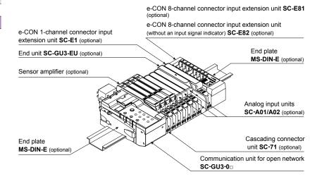
\*If optical communication is to be used in a system that includes models not compatible with optical communication, connect the incompatible models after the SC-GU3-EU. A maximum of 12 units can be connected to the FX-500 / LS-500 series, and a maximum of 16 units can be connected to the other sensor amplifiers.
