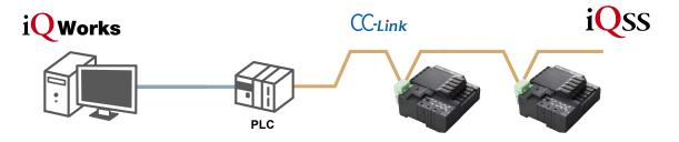
Mitsubishi Electric's iQ Works utility can be used to control digital sensors connected to the **SC-GU3-01**.
