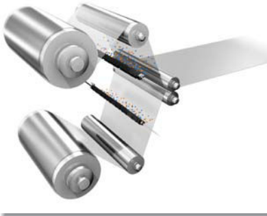
Removing dust while separating TAB protective film
