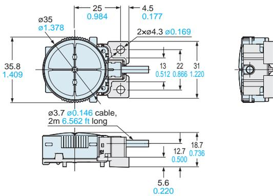
**Assembly dimensions with mounting bracket**
