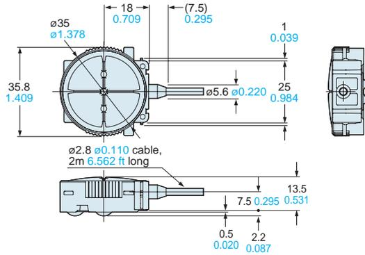
**Assembly dimensions with mounting bracket for MS-SQ4-21**
