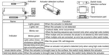
Note: When check the LED light transmitted to the actuator, depending on the angle, yellow lights may separated into green and red
