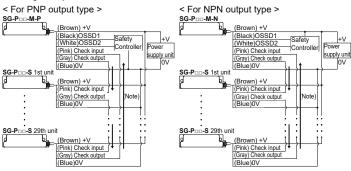
Note: For connecting multiple units, connect the check output line (gray) with the check input line (pink) of the SG-Pao-S sub unit connected next. Connect the check output line (gray) of the SG-Pao-S sub unit connected at the end with the check input line (pink) of the SG-Pao-M standard unit placed at the beginning.
