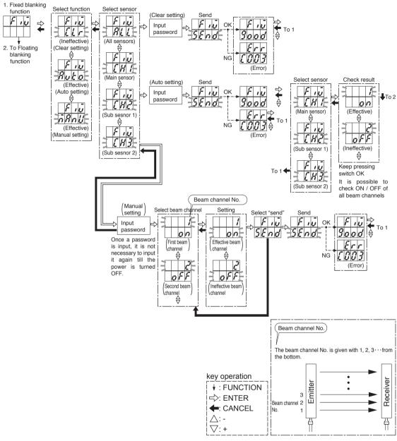
\*: The functional setting for each beam channel is as follows.
