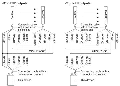
• Connection cable with a connector on one end: 2 pcs./set
