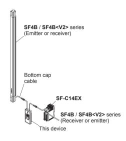
3. Turn ON the power, and set the function with this device. After the power of this device is ON, a total approx. 30 sec. will be taken for data transmission with SF4B / SF4B<V2> series and SF-C14EX. While data transmission, " " lights up in revolving. The safety output 1 / 2 of SF-C14EX series are set to "OFF" while this device has been connected.]
