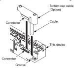
2. Tighten the two M2.6 screws. Tighten to a torque of 0.3N·m or less.
