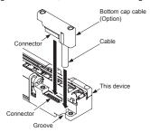
2. Tighten the two M2.6 screws. Tighten to a torque of 0.3N·m or less.
