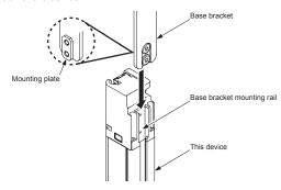
2. With the base bracket in firm contact with the device, tighten the two ultra lowhead hex socket bolts [M5 (length 5mm), opposing faces 3mm] that fasten the base bracket. Tighten to a torque of 3N·m or less
