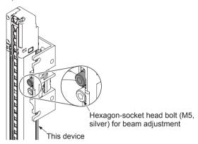
Step 6 Fully tighten the two hexagon-socket head bolts [M5] or the two hex bolts [M6] you partially tightened in step 1.
