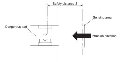
[For use in Europe (EU) (based on EN ISO 13855)] (Also applies to JIS B 9705) (For intrusion perpendicular to the sensing area)
