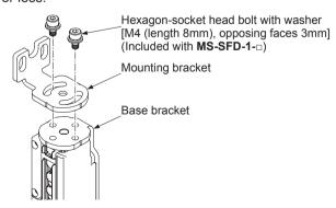
Step 3 Install the beam adjustment mounting bracket on the mounting surface with a hexagon-socket head (purchase separately).
