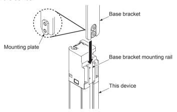
Step 2 With the base bracket in firm contact with the device, tighten the two ultra low-head hex socket bolts [M5 (length 5mm), opposing faces 3mm] that fasten the base bracket. Tighten to a torque of 3N·m or less.
