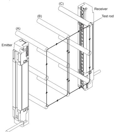
Step 5 While moving the test rod in Step 4, verify that the control output (OSSD 1 / 2) is OFF while the test rod is in the sensing area. In addition, verify that the OSSD indicator of the receiver and the operation indicator of the emitter both light red.
