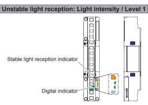
Step 7 If the stable light reception indicator lights green the device is in the stable light reception state.
