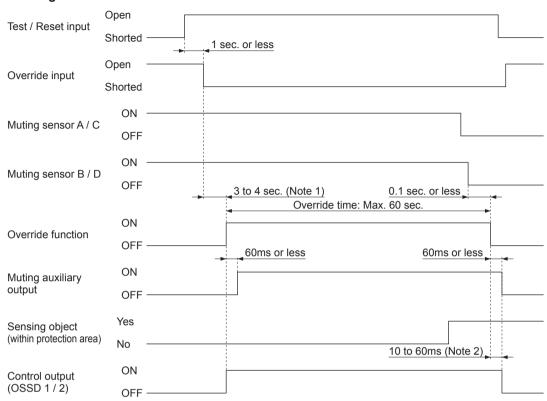
Notes: 1) If the muting indicator does not turn ON after 1 sec. when the muting indicator diagnosis function is valid, the override function is invalid. When the muting indicator diagnosis function is invalid, the muting function is valid 3 sec. after the input conditions of muting sensors A (C) and B (D) are satisfied.
