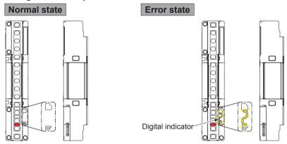
Step 4 Check the upper application indicator and lower application indicator on the emitter, the operation indicator, the upper application indicator and lower application indicator on the receiver, and the OSSD indicator.
