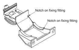
Step 3 Install the intermediate supporting bracket on the mounting surface with two hexagon-socket head bolts [M5 (purchase separately)].
