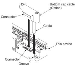
Step 2 Tighten the two M2.6 screws. Tighten to a torque of 0.3N·m or less.
