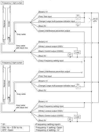
Notes: 1) The orange indicator lights up when the input wire for the large multi-purpose indicator (orange) is connected to the +V terminal, and turns OFF when it is disconnected.
