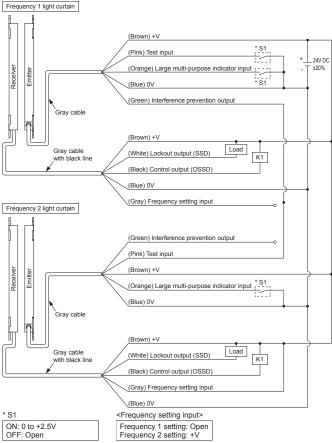
ote: The orange indicator lights up when the input wire for the large multi-purpose indicator (orange) is connected to the +V terminal, and turns OFF when it is disconnected.
