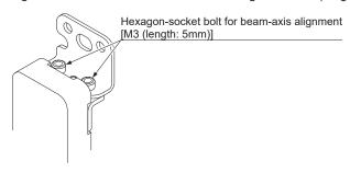
Step 4 Change direction of the part A of multifunctional mounting bracket. And tighten the two of hexagon-socket head bolts for beam-axis alignment M3 (length 5mm)]. The tightening torque should be 2 N•m or less.
