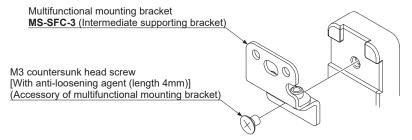
Step 3 Set the multifunctional mounting bracket on the mounting surface using either two hexagon head bolts [M6 (purchase separately)] or four hexagon head bolts [M4 (purchase separately)].
