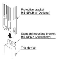
Step 2 Position mounting holes of protective metal Case and standard mounting bracket. And, tighten with two hexagon-socket head bolts [M5 (purchase separately)] on the mounting surface.
