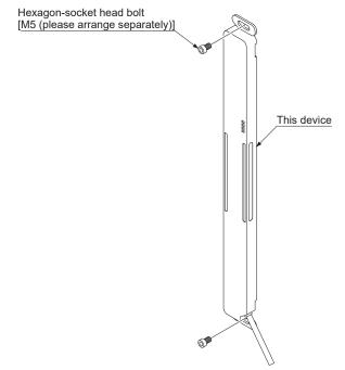
Note: The case of the product is made of resin so the longitudinal dimension is subject to expansion and contraction. When drilling mounting holes, check the drilling locations by positioning the actual product at the installation location.
