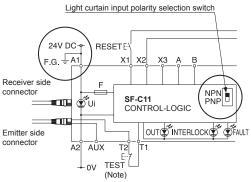
Note: Emission halt occurs when the test (TEST) button is open, and emission occurs when the test (TEST) button is short-circuited. If not using the test (TEST) button, shortcircuit T1 and T2.
