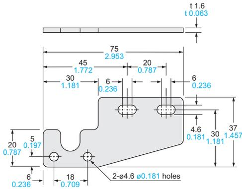
Material: Cold rolled carbon steel (SPCC)
