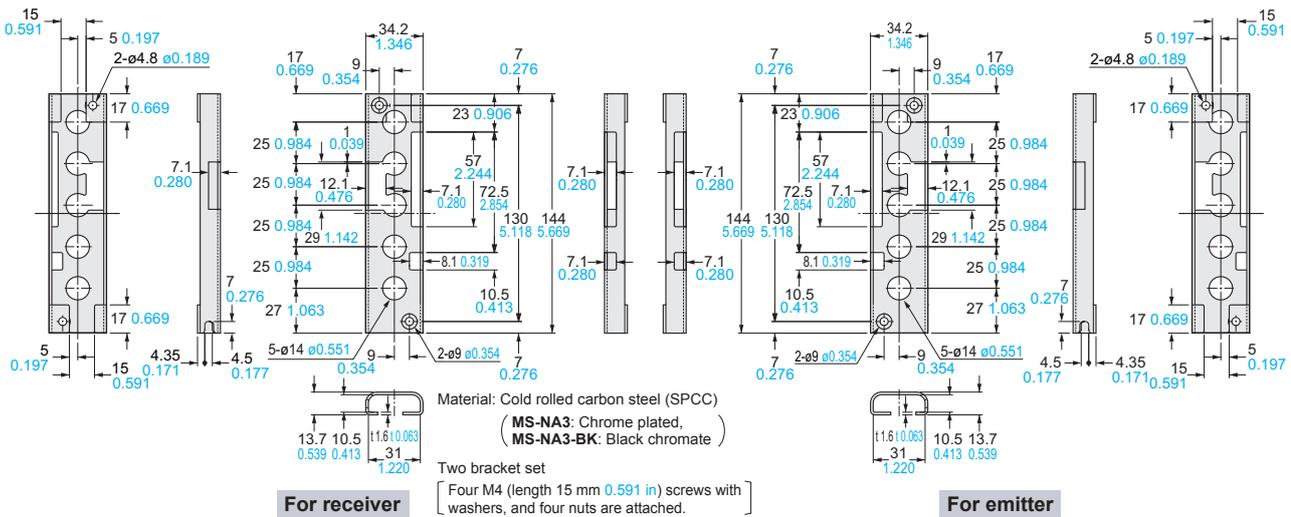
Material: Cold rolled carbon steel (SPCC)
