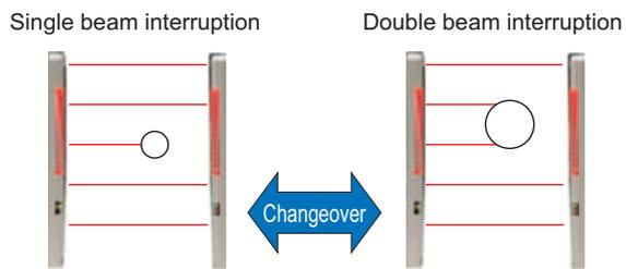
All opaque bodies with  $\varnothing 35$  mm  $\varnothing 1.378$  in or greater will be detected.
