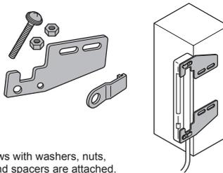
M4 screws with washers, nuts, hooks and spacers are attached.
