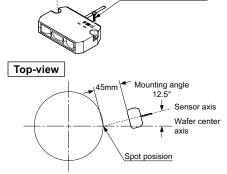
Note: If the wafer center axis and the sensor axis lie along a straight line, detection is not possible. Always mount the sensor at an angle to the wafer.
