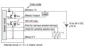
Symbols ... D: Reverse supply polarity protection diode ZD1, ZD2: Surge absorption zener diode Tr1: NPN output transistor Tr2: PNP output transistor
