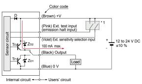
Symbols  $\dots$  D: Reverse supply polarity protection diode ZD1, ZD2: Surge absorption zener diode Tr1: NPN output transistor Tr2: PNP output transistor
