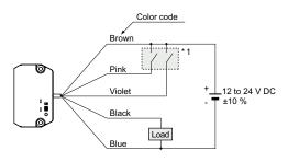
Non-voltage contact or PNP open-collector transistor External test input (emission halt input) 0 to 3 V, or 9 V to +V (26.4 V max.): Emission halt Open, or 4 to 8 V: Emission External sensitivity selection input 0 to 3 V, or 9 V to +V (26.4 V max.): Input ON Open, or 4 to 8 V: Input OFF
