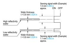
From the above, for determining the position of the wafer from the sensing signal, calculate the center position of the signal's ON region, while taking into consideration the response time.
