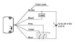
Non-voltage contact or NPN open-collector transistor • External test input (emission halt input) 0 to 3 V, or 9 V to +V (26.4 V max.): Emission halt Open, or 4 to 8 V: Emission External sensitivity selection input 0 to 3 V, or 9 V to +V (26.4 V max.): Input ON Open, or 4 to 8 V: Input OFF
