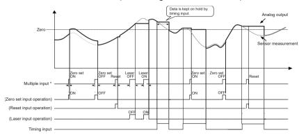
• NORMAL measurement (with timing mode set to "One-shot")
