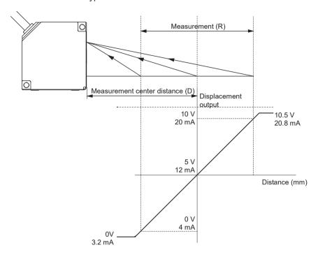
\*1 In the figure above, analog output setting is used as the initial setting.
