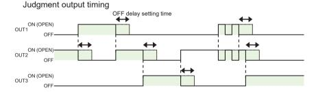
The solid lines shows OFF setting actions. OFF timing will be delayed according to the OFF-delay set time as shown by the dotted lines.
