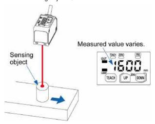
**3.** If the measured value falls within the range of the threshold set in "4.1.3 2-point Teaching (Normal Sensing Mode)", the output operation indicator will light up.
