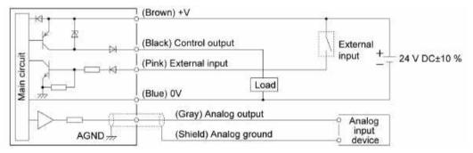
(Note 1) Insulate unused terminals to avoid error input or short circuit.
