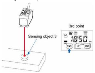
6. The threshold value 1 and threshold value 2 will be set and teaching will be completed. If the difference between the teaching results for the sensing objects 1 to 3 is equal to or larger than the shift amount, "good" will be displayed on the digital display. Then the desired threshold value is displayed and the teaching indicator turns OFF.
