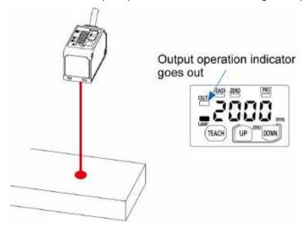
2. Insert a sensing object. Check that the measured value on the digital display fluctuates.
