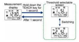
When adjusting the threshold value just switched over, press the UP key or DOWN key on the measurement display and adjust the threshold value.
