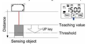
4. If the difference between the teaching results for the background object and the sensing object is equal to or larger than the shift amount, "good" will be displayed on the digital display. Then the desired threshold value is displayed and the teaching indicator turns OFF.
