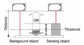
4. If the difference between the teaching results for the background object and the sensing object is equal to or larger than the shift amount, "good" will be displayed on the digital display. Then the desired threshold value is displayed and the teaching indicator turns OFF.
