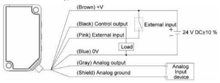
(Note 1) Insulate unused terminals to avoid error input or short circuit.
