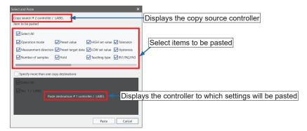
3. The settings can be pasted to multiple controllers at one time. Select the Specify more than one copy destination check box and select applicable controllers.
