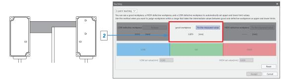
**3.** Measure a HIGH defective workpiece and click **Fix the measured value**.
