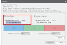
2. Measure the second workpiece and click the Fix the measured value button for the second workpiece.
