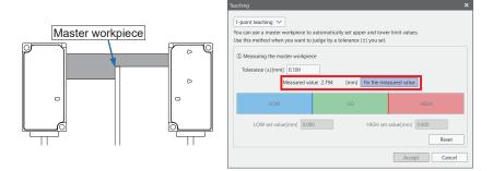
3. The HIGH and LOW set values will be set. By entering a numerical value, you can adjust the HIGH or LOW set value within the range (between the HIGH and LOW set values).
