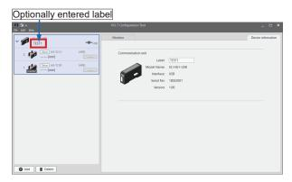
Note: Labels of communication units are managed by the tool software in the PC. If the tool software is reinstalled or the communication unit is connected to another PC, the set label will not be retained.
