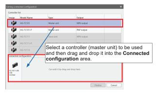
4. After selecting the master unit, select a slave unit and then drag and drop it into the Connected configuration area.
