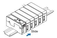
3. Attach end plates MS-DIN-E (optional) with the flat side facing in so as to enclose the connected units at the ends.
