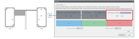
**4.** The HIGH and LOW set values will be set. By entering a numerical value, you can adjust the HIGH or LOW set value within the range (between the HIGH and LOW set values).
