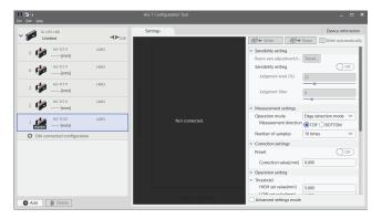
7. After all the controllers to be used have been set up, select Save as from the File menu and save the configuration file.
