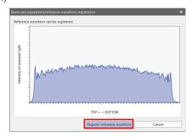
When the registration is completed, the message "Reference waveform has been registered" will be displayed. Clicking **OK** closes the message window.
