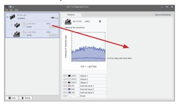
**6.** The monitor screens of the two controllers will be displayed in the **Monitor** tab window.
