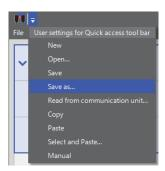
2. Clicking Save as displays a tick mark on the left of Save as and adds the pight side of HG-T Configuration Tool.
