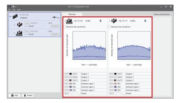
WUME-HGTCT-3 8-3 · When multiple controllers are monitored, the display of received light waveforms can be reversed. Clicking the Reverse the waveform check box in each monitor screen reverses the display of the received light waveform.
