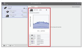
5. Click the second controller to be monitored and drag and drop it into the area in the Monitor tab window in the same way as above.
