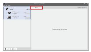
Click the first controller to be monitored and drag and drop it into the area in the Monitor tab window.
