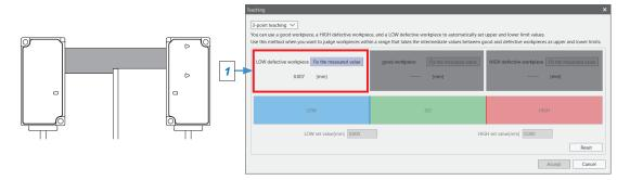
2. Measure a good workpiece and click Fix the measured value.
