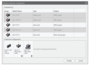
3. Edit the connection configuration by adding or deleting controllers. After editing the connection configuration, click **Finalize** to reflect the configuration in the connected units window.
