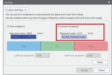
3. The HIGH and LOW set values will be set. By entering a numerical value, you can adjust the HIGH or LOW set value within the range (between the HIGH and LOW set values).
