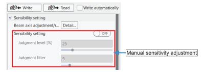
1. Slide the Sensitivity setting switch from OFF to ON. (Default: OFF)
