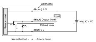
Note: Please carry out the wiring carefully since protection circuit against reverse power supply connection is not incorporated.
