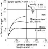
Correlation between sensing object size and sensing range As the sensing object size becomes smaller than the standard size (iron sheet  $40\times40\times t$  1 mm  $1.575\times1.575\times t$  0.039 in), the sensing range shortens as shown in the left figure.
