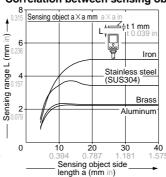
As the sensing object size becomes smaller than the standard size (iron sheet  $25 \times 25 \times t$  1 mm  $0.984 \times 0.984 \times t$  0.039 in), the sensing range shortens as shown in the left figure.
