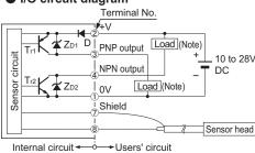
Note: Connect the surge absorption diode in parallel with the load when the conductance coil such as relay is connected or taken off.
