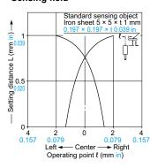
The graph on the left is plotted with the sensitivity adjusted so as to just detect a 5 × 5 × t 1 mm  $0.197 \times 0.197 \times t \ 0.039$  in iron sheet placed at a distance of 1.0 mm 0.039 in.
