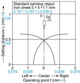
The graph on the left is plotted with the sensitivity adjusted so as to just detect a 5 × 5 × t 1 mm  $0.197 \times 0.197 \times t \ 0.039$  in iron sheet placed at a distance of 0.6 mm 0.024 in.
