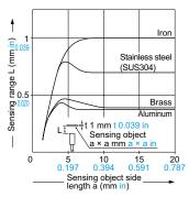
As the sensing object size becomes smaller than the standard size (iron sheet 5 × 5 × t 1 mm 0.197 × 0.197 × t 0.039 in), the sensing range shortens as shown in the left figure
