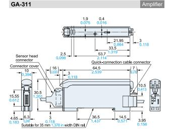
Note: The front view shows the sensor head connector and quick-connection cable connector attached.
