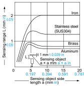
As the sensing object size becomes smaller than the standard size (iron sheet 10 × 10 × t 1 mm 0.394  $\times$  0.394 × t 0.039 in), the sensing range shortens as shown in the left figure.
