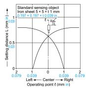
The graph on the left is plotted with the sensitivity adjusted so as to just detect a 5 x 5 x t 1 mm  $0.197 \times 0.197 \times t \ 0.039$  in iron sheet placed at a distance of 0.8 mm 0.031 in.
