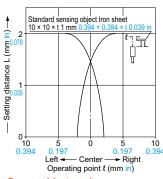
The graph on the left is plotted with the sensitivity adjusted so as to just detect a 10 × 10 × t 1 mm × 0.394 × t 0.039 in iron sheet placed at a distance of 2.0 mm 0.079 in.
