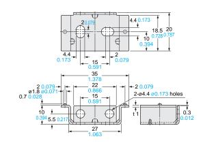
Material: Cold rolled carbon steel (SPCC) (Uni-chrome plated)
