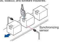
Notes: 1) FD-L52 fiber head (high precision type) or FD-L53 fiber head (extremely small spot type) is recommended for applications in which specular objects, having a high reflective index are to be detected, e.g., evaluating if metal objects are plated or not.
