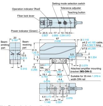
MS-DIN-3 Amplifier mounting bracket (Accessory for amplifier)
