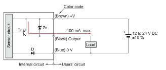
Symbols ... D : Reverse supply polarity protection diode ZD: Surge absorption zener diode
