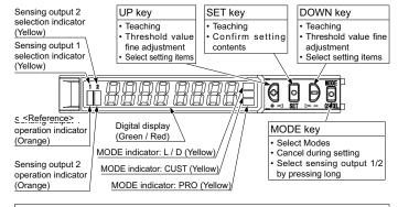
Pressing down SET key + MODE key for 3 sec : Set key lock or Release key lock
