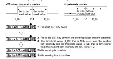
Notes 1) The shift amount of 10% is an initial value. The shift amount can be set in PRO mode. Furthermore, the shift value can be set in incident light amount. For setting method, refer to <PRO6> in \*PRO MODE OPERATION MANUAL.\*
