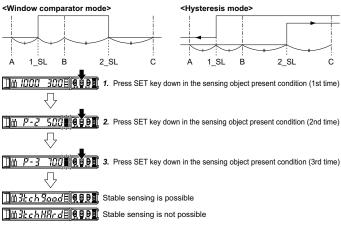
Note: If the value after setting exceeds the maximum (minimum), the maximum (minimum) sensitivity will be set.
