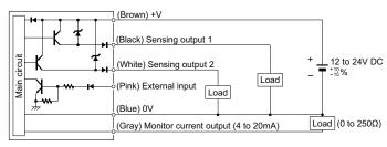
Note: Make sure to insulate the ends of the unused lead wires
