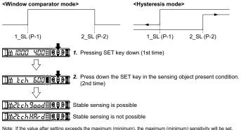
Note: If the value after setting exceeds the maximum (minimum), the maximum (minimum) sensitivity will be set.
