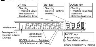
Pressing down SET key + MODE key for 3 sec : Set key lock or release key lock
