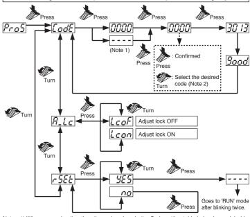
Notes: 1) When any code other than the codes given in the Code setting table below is used, ' - ' is displayed. The factory setting is '0004'.
