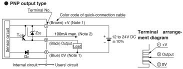
Notes: 1) The quick-connection sub cable does not have +V (brown) and 0V (blue) The power is supplied from the connector of the main cable 2) 50mA max., if five, or more, the amplifiers are connected in cascade.
