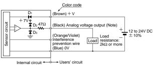
Note: The output is not incorporated with a short-circuit protection circuit. Do not connect it directly to a power supply or a capacitive load.
