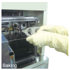
Vacuum baking for the reduction of outgas
