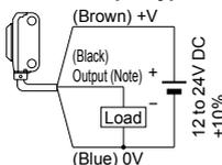
Note: The thru-beam type sensor emitter does not incorporate the output.
