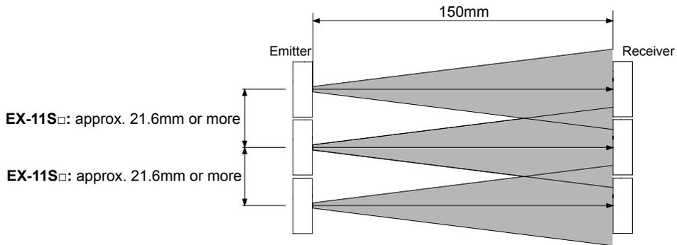
**Thru-beam type: EX-11SE□, parallel deviation diagram (typical)**
