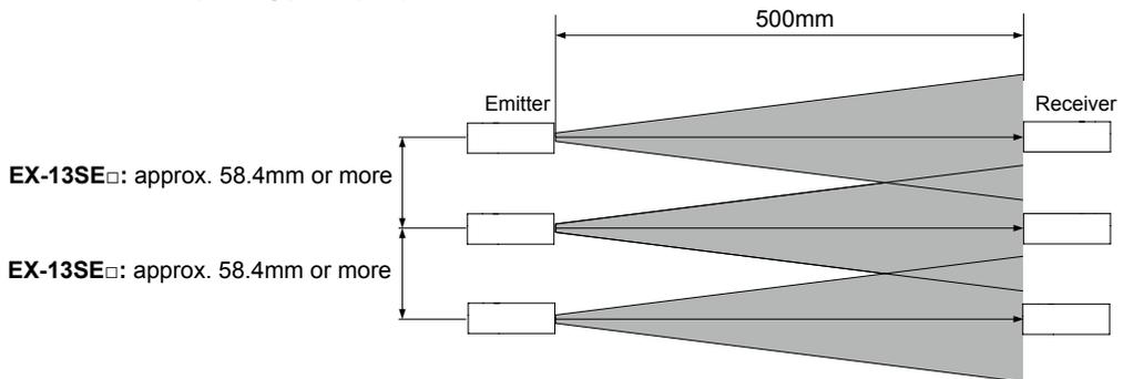
**Thru-beam type: EX-19S□, parallel deviation diagram (typical)**
