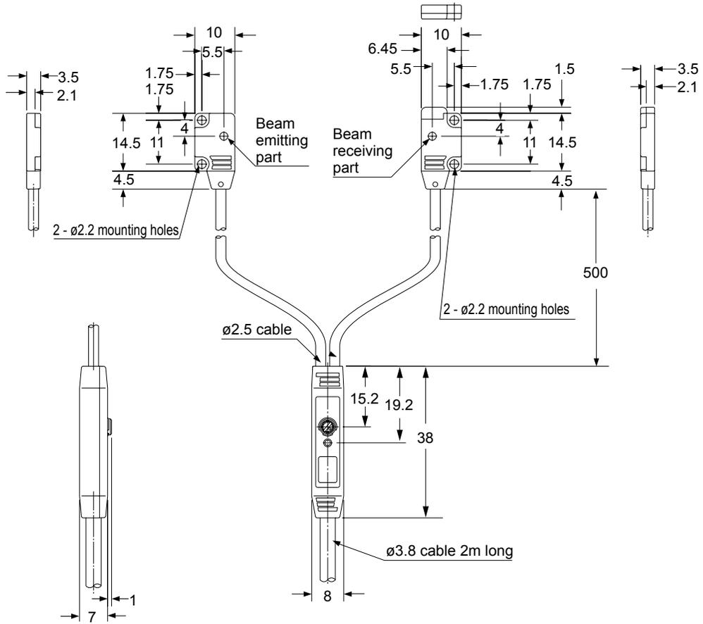
**Thru-beam side sensing type with operation mode switch on bifurcation: EX-15E, EX-17E**
