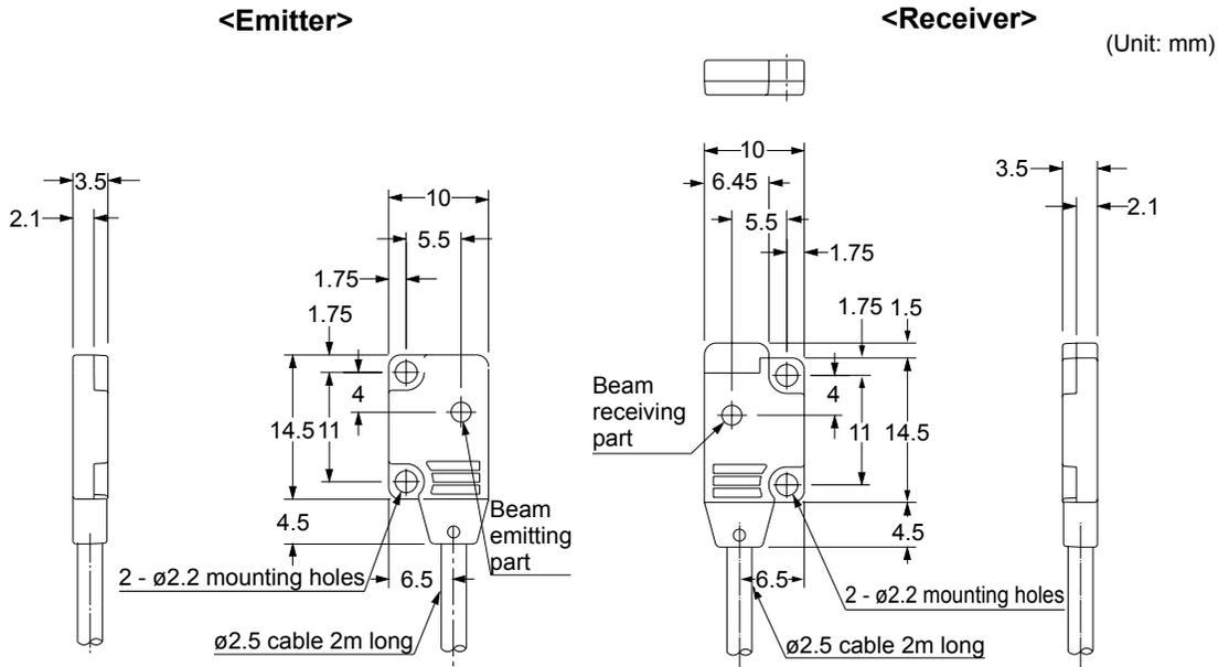
Thru-beam side sensing type: EX-11E□, EX-13E□, EX-19E□
