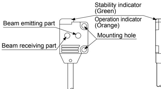
**Thru-beam front sensing type with operation mode switch on bifurcation:
