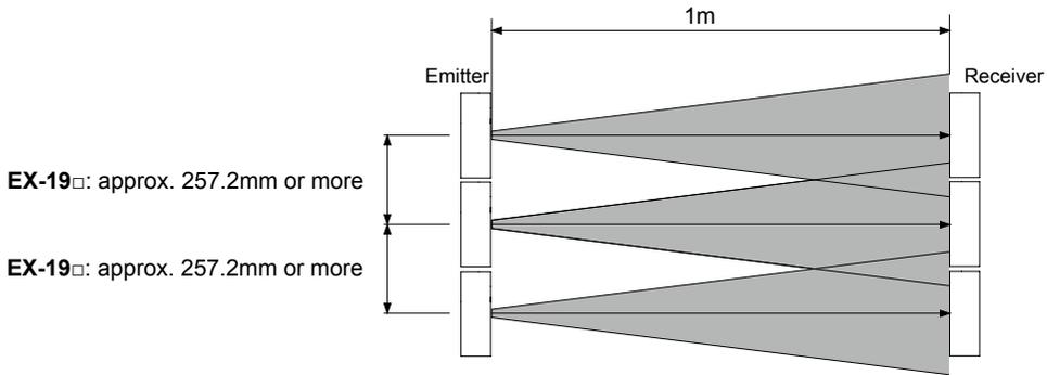
**Thru-beam type: EX-19E□, parallel deviation diagram (typical)**
