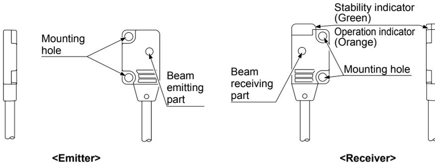
Thru-beam side sensing type: EX-11E□, EX-13E□, EX-19E□
