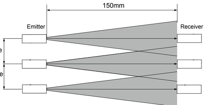
**Thru-beam type: EX-13□, EX-17□ parallel deviation diagram (typical)**
