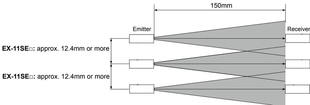
**Thru-beam type: EX-13S□, parallel deviation diagram (typical)**
