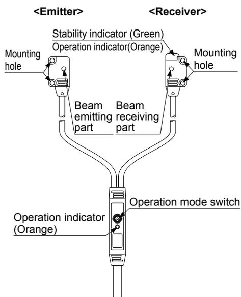
**Thru-beam side sensing type with operation mode switch on bifurcation:
