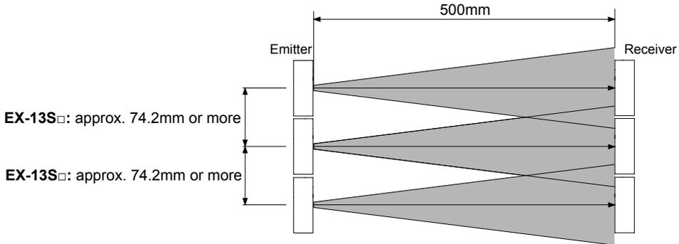
**Thru-beam type: EX-13SE□, parallel deviation diagram (typical)**
