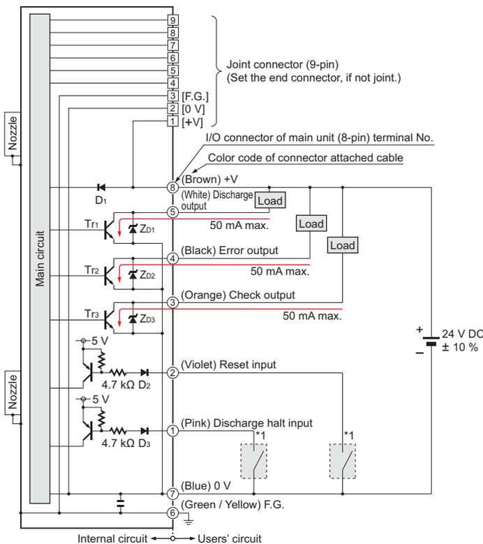
Symbols ... D1: Reverse supply polarity protection diode
