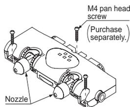
**Adjusting the air blowing direction**
