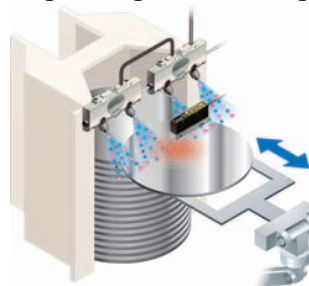
Surface potential measurement during loading and unloading
