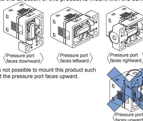
Note: It is not possible to mount this product such that the pressure port faces upward.
