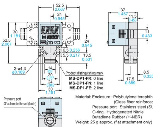
Material: Enclosure...Polybutylene terephthalate (PBT) (Glass fiber reinforced)
