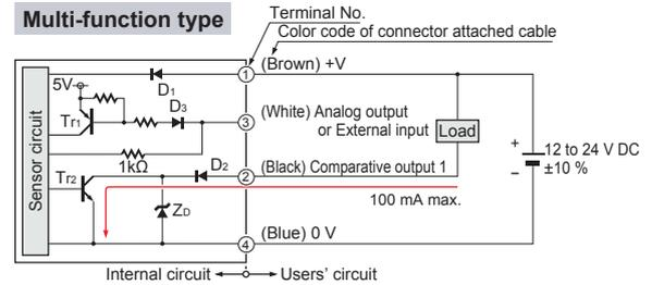
Symbols... D1 to D3 : Reverse supply polarity protection diode
