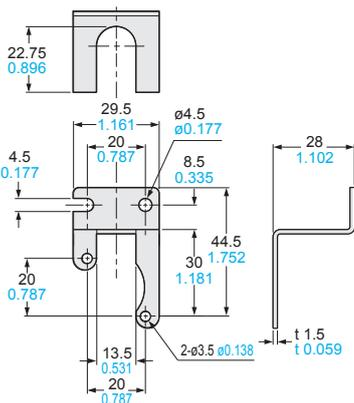
Material: Cold rolled carbon steel (SPCC)
