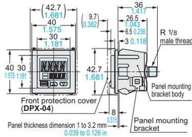
Note: The panel thickness should be 1 to 32 mm 0.039 to 1.260 in.
