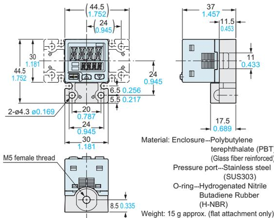
Material: Enclosure...Polybutylene terephthalate (PBT) (Glass fiber reinforced)
