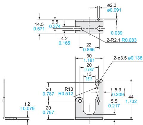
Material: Cold rolled carbon steel (SPCC)
