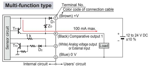
Symbols... D1, D2 : Reverse supply polarity protection diode
