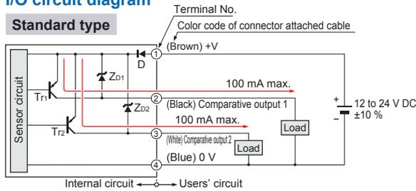
Symbols... D : Reverse supply polarity protection diode
