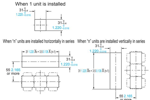
Note: The panel thickness should be 1 to 6 mm 0.039 to 0.236 in.
