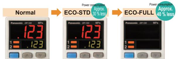
Current consumption for 24 V power supply: **35 mA or less** (Normal), **25 mA or less** (ECO-STD), **20 mA or less** (ECO-FULL)
