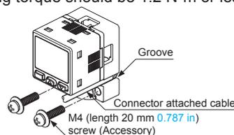
Note: Take care that if the cable with connector is sticking out of the side groove of this product when mounting, the cable may be disconnected.
