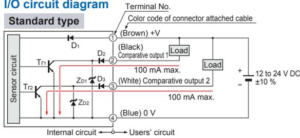
Symbols... D1 to D3 : Reverse supply polarity protection diode
