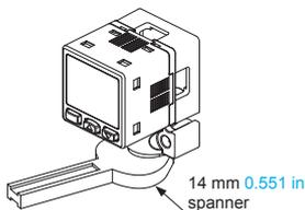
Note: Do not tighten the pressure port by holding the product with the spanner. It may cause the product breakage.
