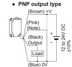
Note: This is sensing mode selection input. Wire the sensing mode selection input to either 0V (blue) or +V (brown), and select the sensing mode (BGS/FGS function)
