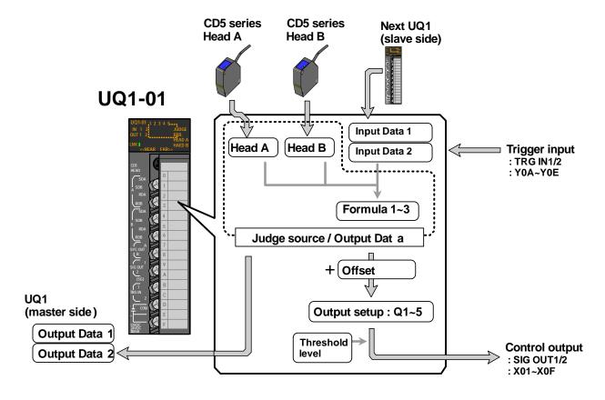
Chart above shows the data flow of the UQ1-01 for the CD5 series UQ1-02 version is for the CD33 Series. The same principle applies
