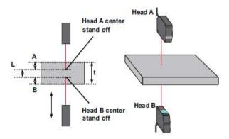
For example, when the thickness of the object is 10mm and "A+B" is 9.2mm, set the formula as follows. Set the "Fixed value" as "0.800" (L=t-A-B then 10mm - 9.2mm = 0.8mm).
