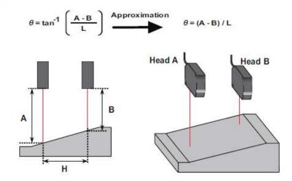
When the distance between two sensor heads is 80mm for example, the formula is as follows.
