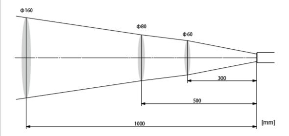
The fields of view stated above are measurement diameters with an optical response of 90%.
