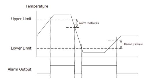
Alarm output turns on when the measured temperature exceeds the upper alarm limit.
