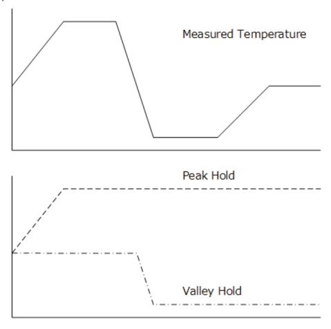
Use the [System command] "Reset hold" to reset the held temperatures.
