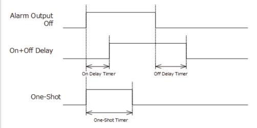
When [Alarm timer function] is set to [Delay], the output is delayed for the time set with [On delay time] and [Off delay time] as shown with "Delay" in the above diagram.
