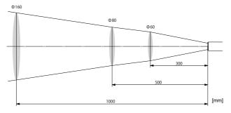
The optical resolution values stated in "Field of View" are at minimum 90% energy. The size of measuring object should be sufficiently lager than the field of view (spot size) shown in the above illustration
