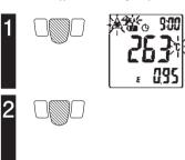
Pressing the (MEASURE) button to turns ON the power supply. A laser beam emitted and the measurement starts. In the Normal Measurement mode, the units takes measurement while
