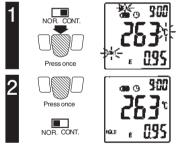
When the (MEASURE) button is pressed while the DIP switch is adjusted to the CONT. side (Refer to "DIP switch setting" in page 7.), "CONT" is lit on LCD and continuous measurement is started. Measurement continues even if releasing the (MEASURE) button.
