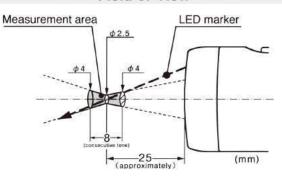
The measurement area depends upon 90% energy limit of optical responce. The object size should be larger than the above area. The maximum spot size is  $\phi 4$ IIII in the above measuring area.
