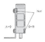
OScrew tightening torque should be 8kgf ·cm(0.8 Nm)max.
