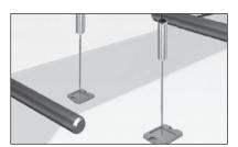
[Detection of chips/cracks in liquid crystal glass]
