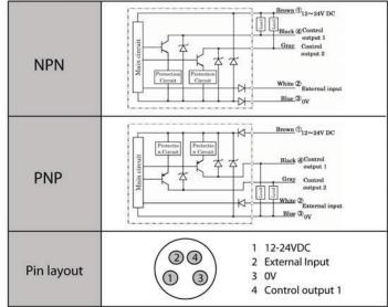
Gray line (Control output 2) is only for the 2 output type (D3RF-TD).
