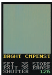
Screen after brightness irregularity correction (There is no irregularity in brightness)
