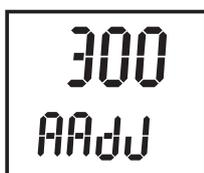
The adjusted value are effective after the both of L and H value are set and stored. When AADJ mode on, AADJ is displayed as sub indication. The measuring value is output according to the setting value previously stored, if the setting of L and H value are stored in EXIT mode with AADJ mode on. In this process, AADJ is also displayed as sub indication.
