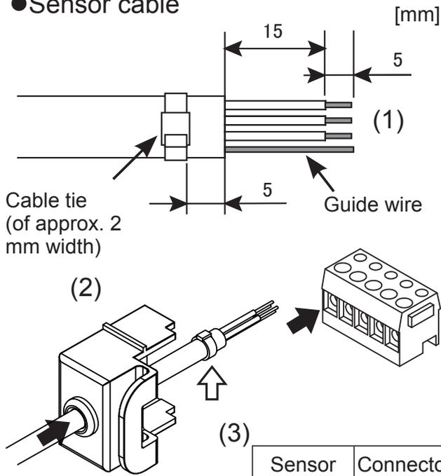
When you cut the sensor cables, ensure to perform end treatment and connection of the cables.
