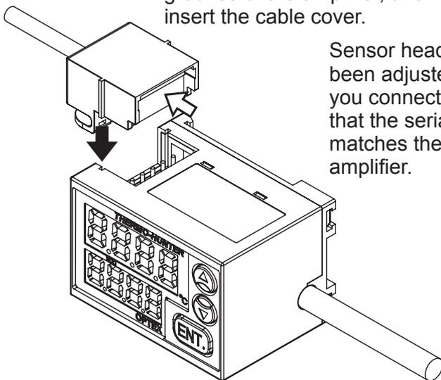
Sensor head and amplifier has been adjusted in one set. When you connect both, make sure that the serial number of cable matches the serial number of amplifier.
