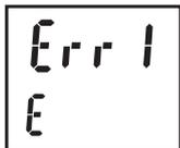
In the TECH mode, if the automatically calculated emissivity rate is outside the setting range (0.1 to 1.2), an error (Err1) occurs. In this case, the emissivity rate cannot be set in the TECH mode. Set it in the  $\epsilon$  mode again.
