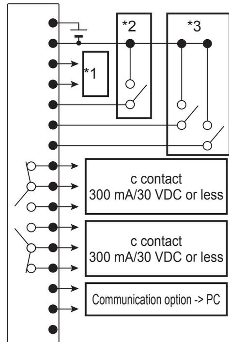
\*1 Connect to the 4-20 mA input of an analog device.
