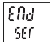
Flashing / Button operation is not possible
