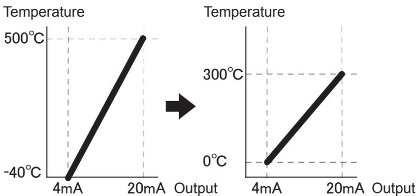
\* The minimum width of output range is 100°C. You cannot set it to less than 100 °C.
