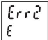
In the TECH mode, if the temperature measurement value calculated with the automatically calculated emissivity rate is outside the measurement temperature range, an error (Err2) occurs. In this case, the emissivity rate cannot be set in the TECH mode. Set it in the  $\epsilon$  mode again.
