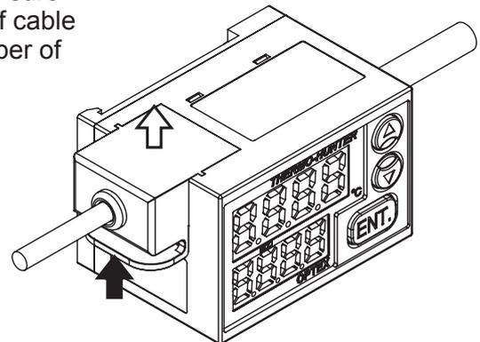
Amplifier is not a protective structure. When you connect the output cable and the sensor cable, make sure that the water or oil does not penetrate to amplifier along the cable. When used in such an environment where water or oil might get in to the amplifier, please use optional protective case. (Equivalent to IP65)
