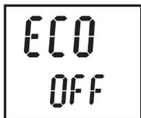
You can reduce consumption current by turning off the display during normal measurement.
