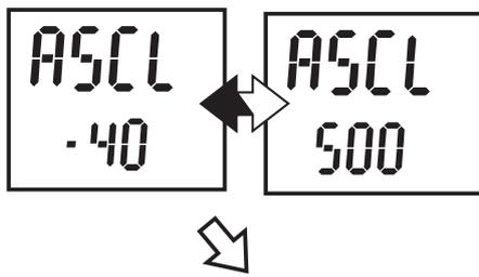
You can change the temperature range of analog output (4 - 20 mA) within the measurement temperature range.
