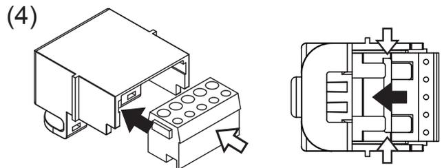
○ Connecting the sensor cables
