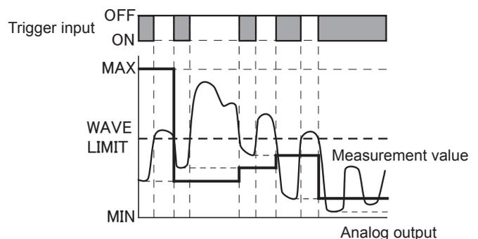
\* After the power is turned on and before the first trigger is input, the minimum value (4 mA) is output in the MAX, P-P and SAMPLE settings and the maximum value (20 mA) in the MIN setting. Sampling starts at the first trigger input, and the analog output control starts from the second trigger input.
