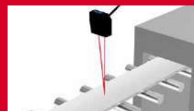
Aluminum material thickness measurement
