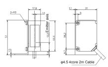
■ Connector type with standard bracket BGS-HL-A
