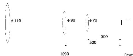
The optical resolution values stated in "Field of View" are at minimum 90% energy. The size of measuring object should be sufficiently larger than the field of view (spot size) shown in the above illustration.
