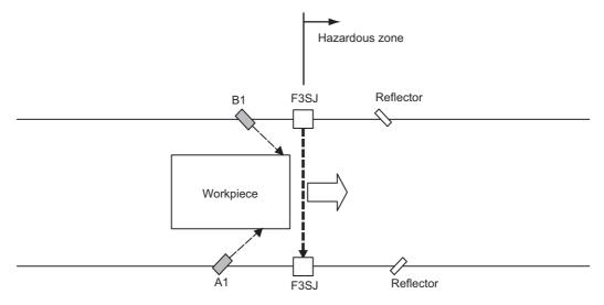
When muting sensors A1 and B1 are turned ON in this order, the muting function is enabled. In this state, the safety function of the F3SJ is disabled.
