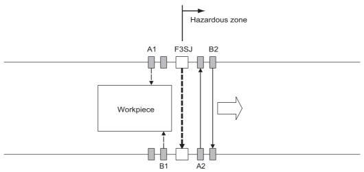
When muting sensors A1 and B1 are turned ON in this order, the muting function is enabled. In this state, the safety function of F3SJ is disabled.
