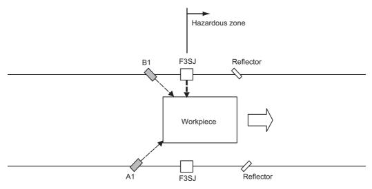
The F3SJ is blocked but the safety function is disabled by the muting function, and safety outputs 1 and 2 are turned ON.
