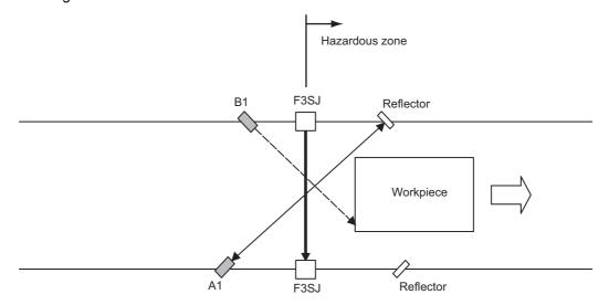
Muting sensor A1 is turned OFF, the muting function is released, and the safety function of the F3SJ is enabled.
