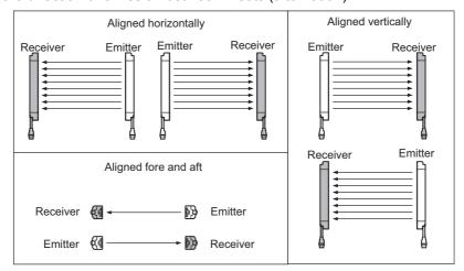
If 2 sets are installed near each other, reflection from the surfaces may cause mutual interference.
