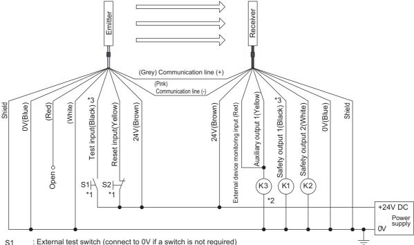
S2 : Lockout reset switch (connect to 24V if a switch is not required)
