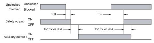
Ton: Response time of safety output's OFF to ON, Toff: Response time of safety output's ON to OFF Response time p.12
