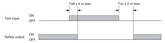
Ton: Response time of safety output's OFF to ON, Toff: Response time of safety output's ON to OFF Response time p.12
