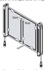
Confirm that hazardous parts should stop while the machine is operating, as shown below.
