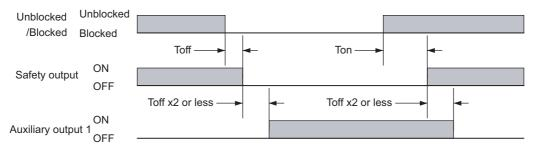
Ton: Response time of safety output's OFF to ON, Toff: Response time of safety output's ON to OFF See p.12 for response time 儿到
