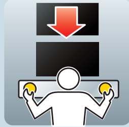
Safe operation with two-hand control
