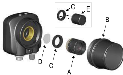
Figure 12. C-Mount Lens Model Components
