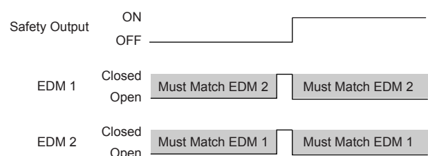
Figure 92. Timing logic: Two-channel EDM status, with respect to Safety Output
