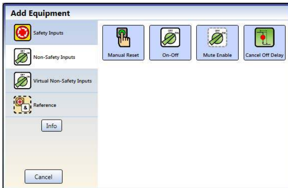
Figure 11. Non-Safety Inputs (Virtual Non-Safety Inputs available only from the Functional View)
